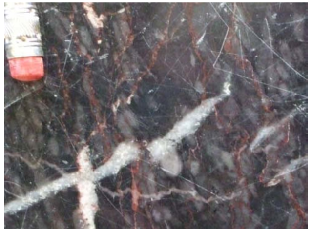
Ashburton Marble, used as a building stone at County Hall, Topsham Road, Exeter
