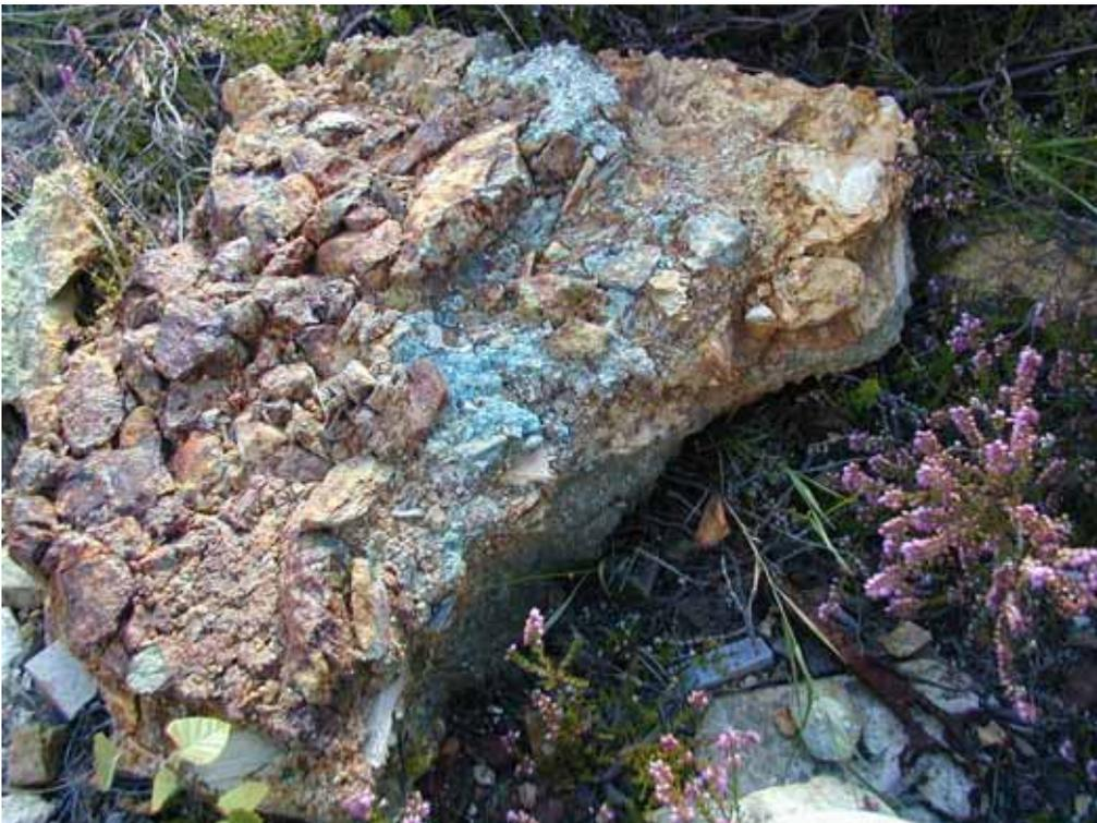
Mine dumps on Devon Great Consols Main Lode at Wheal Anna Maria showing traces of copper mineralisation (blue crusts formed due to the weathering of primary copper sulphide mineralisation).
