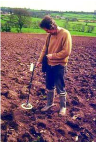
Plate 6: Magnetic Susceptibility survey on the Blackdown Hills in East Devon (© Frances Griffith)
