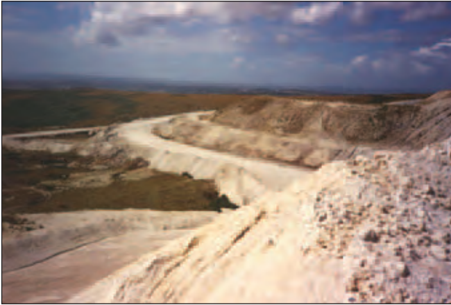
Terraced tipping, Lee Moor.
